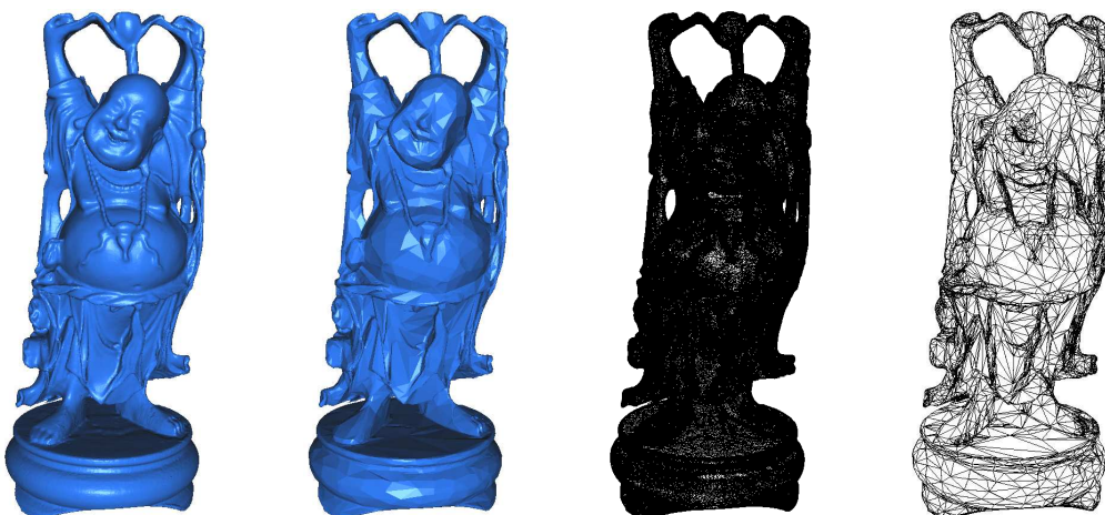
Figure 5: Example of geometric mesh simplification for visualisation purposes. LEFT: original geometry and decimated geometry, RIGHT: original mesh (542,549 vertices) and corresponding decimated mesh (73,896 vertices) - geometry courtesy of INRIA-
