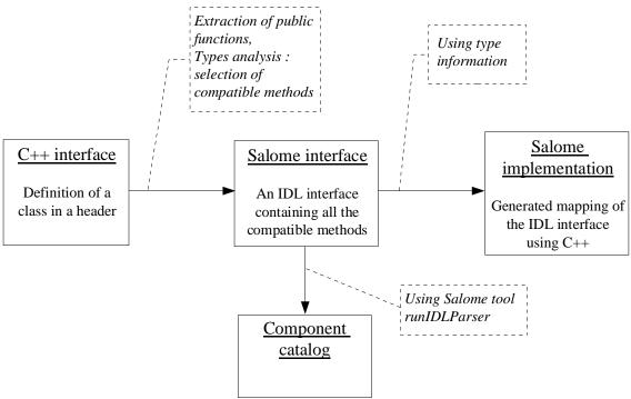
After these operations, the generated files are inserted in a template Salome module (basically a clone of the CALCULATOR component described in ...). We obtain that way a full module ready for compiling.
