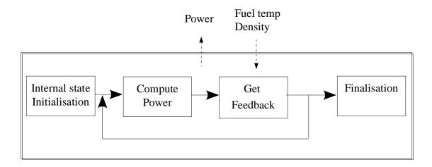
It is designed to exchange MED objects: export of the mesh used for computation, and the neutronic power field, and import of fuel temperature and moderator density fields for thermal-hydraulic feedback.
